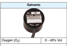
A specific electro chemical sensor for oxygen monitoring.
