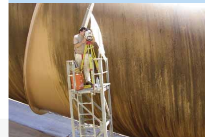
Measuring method with theodolite
